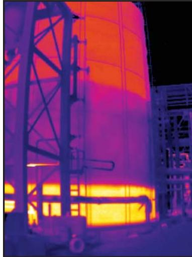
Two silos are being filled, on alternate days, with lime from a kiln. The tank on the right had been filled the previous day while the one on the left was being filled with hot product at the time the image was taken.
