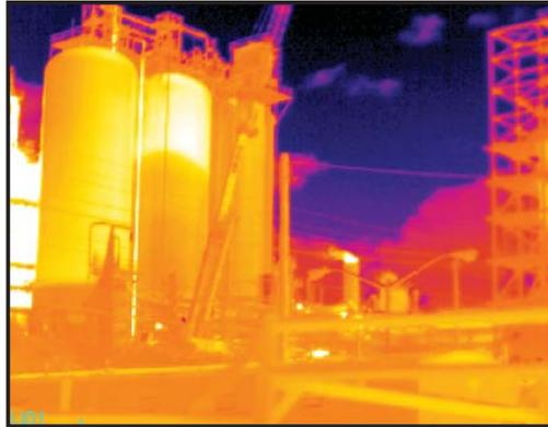
Sludge completely covers the man-way opening in this tank in a paper mill. Anticipating this condition will result in maintenance strategies that are safe and cost effective.
