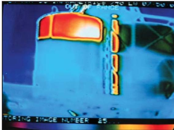
Thermography is an important, cost-effective tool to verify or locate tank levels. A straightforward gas/liquid interface is shown here.
