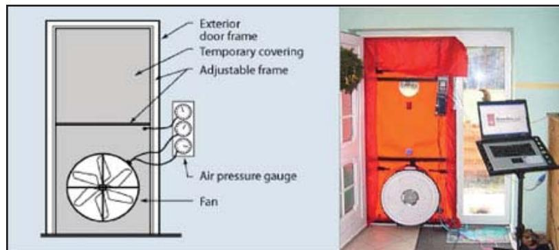
Figure 9: A blower door can help to determine how air tight a building is and to ensure that air sealing work is effective.
