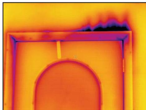
Figure 5: Infiltration around exterior door trim
