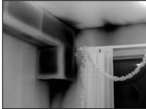
Figure 7: Exhaust fan duct lacks proper insulation
