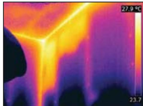
Figure 4: Internal Walls with collapsed/settled insulation
