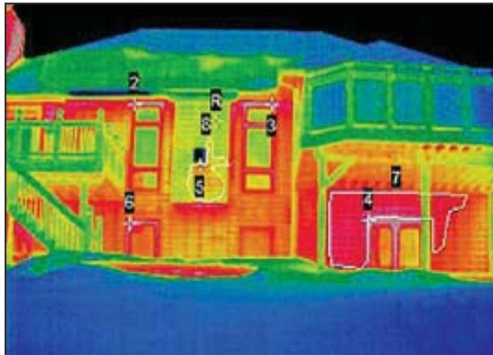
A building is a complex assembly of parts and thermal imaging is very effective at inspecting underlying problems without actually having to tear into the infrastructure. A thermographic inspection provides useful information about a building's envelope such as air in-leakage, moisture ingress, thermal bridges, cavity wall insulation, ceiling/wall junctions and energy efficient windows.
