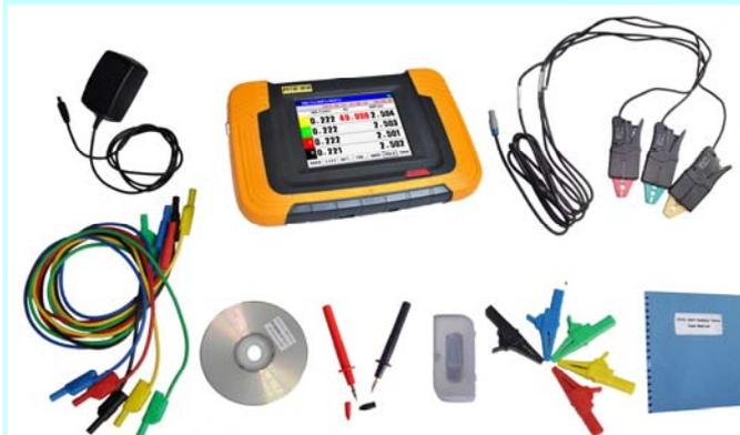
**PITE 3561** includes standard parts of 1 carrying case, 3 color-coded current clamps (example of CC-5A shown above), 1 user manual, 5 alligators, 1 USB drive, 2 voltage probes, 1 software CD, 5 voltage testing leads and 1 power adaptor.
